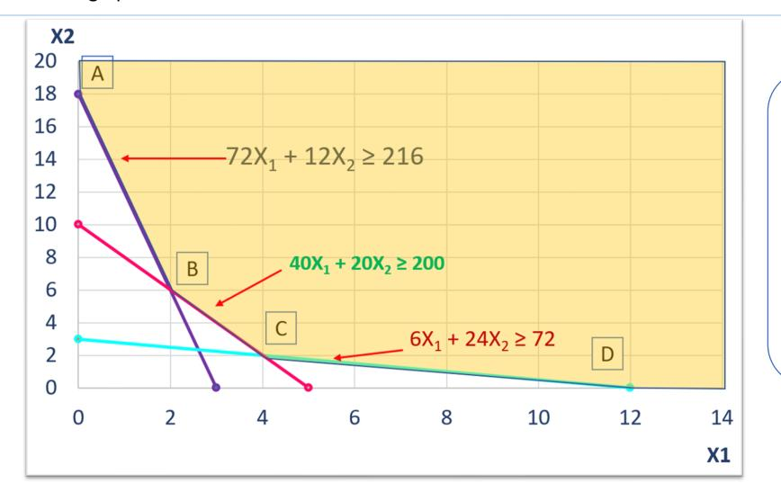
All constraints are greater than or equal to (≥) type. Hence, feasible region should be above (to the right of) all constraints. The vertices of the feasible region are A,B,C & D.
