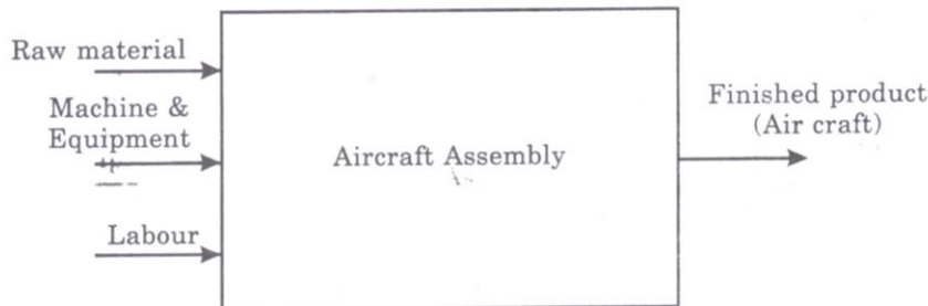
Exhibit 9.3 : Fixed Position Layout or Static Layout
